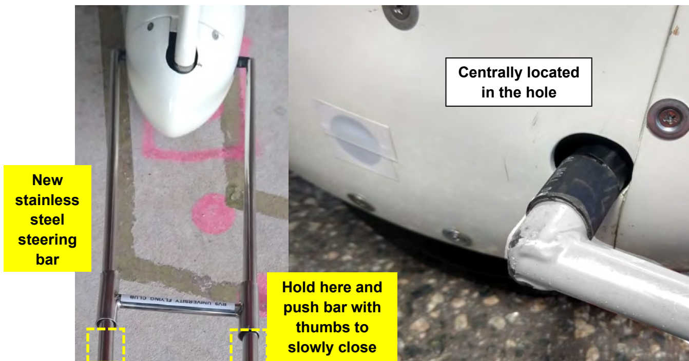
Figure 31 – Steering bar in the attached and closed position. Do not push or pull the aircraft with the steering bar! Only push or pull on the root of the propeller blade.
