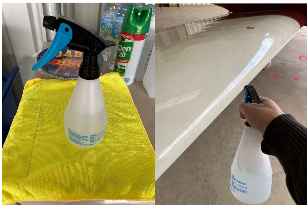
Figure 47 –Clean all of the leading edges.
