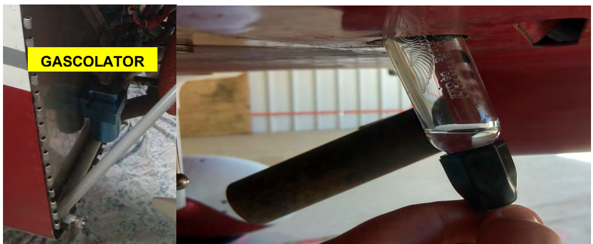
Figure 21 – Hold fuel tester with a slight backward angle to sample the gascolator
