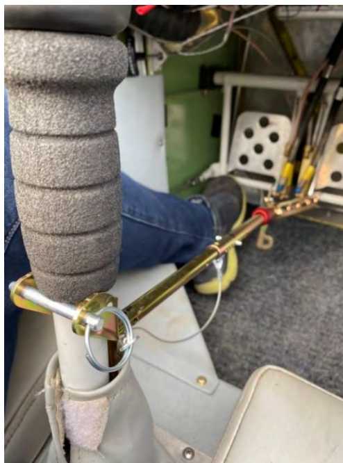
Figure 45 – Control lock installed. Move the stick sheath out of the way to install it properly
