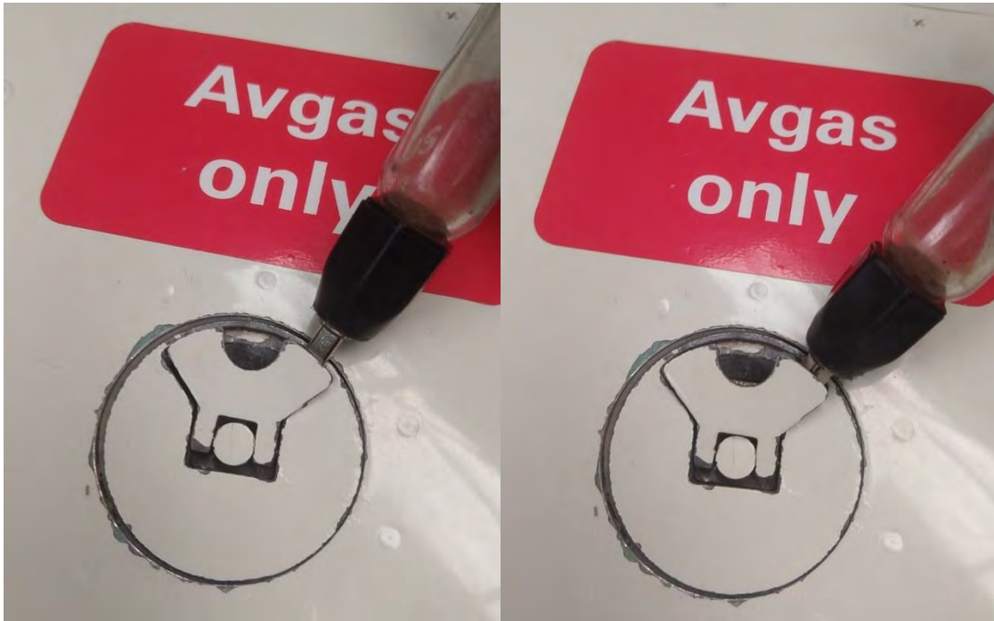
Figure 35 – Carefully insert the flathead of the fuel tester and twist to help lift the flap.
