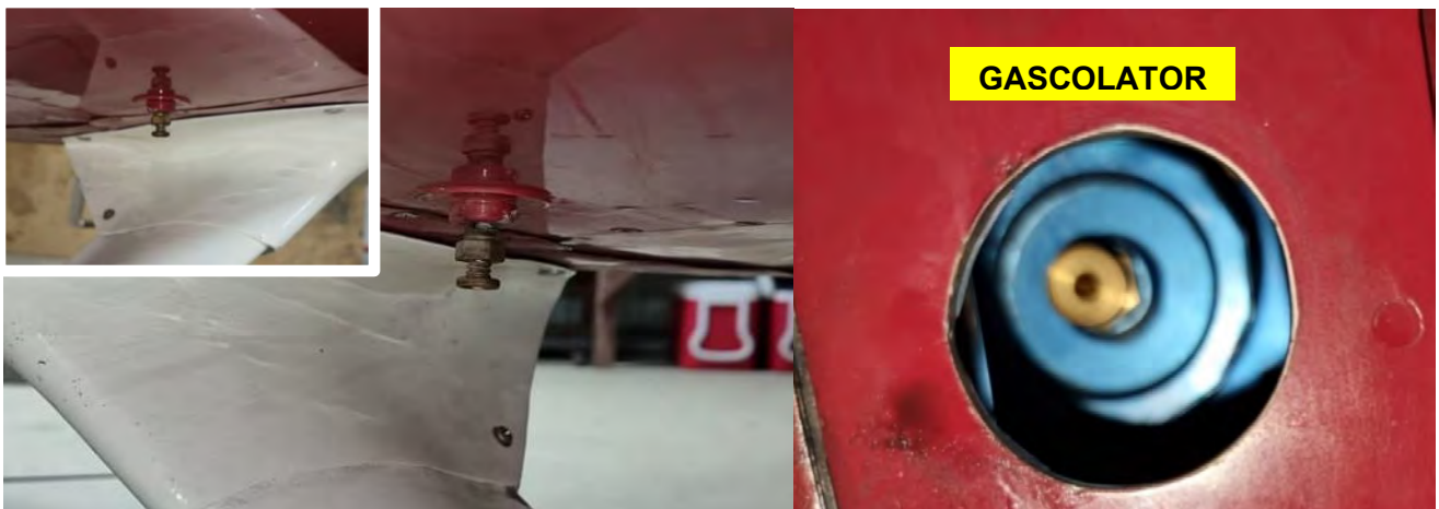
Figure 22 – All three fuel drains are of the same type
