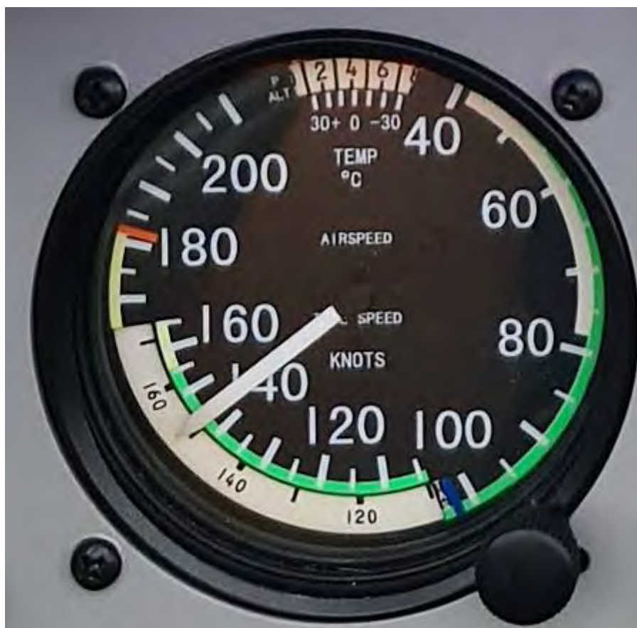
Figure 3 – LAT Analogue Airspeed Indicator with True Airspeed slide rule (to use true airspeed set pressure altitude opposite outside air temperature)
