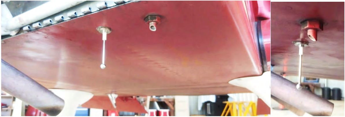
Figure 20 – Port wing fuel vent next to the transponder aerial
