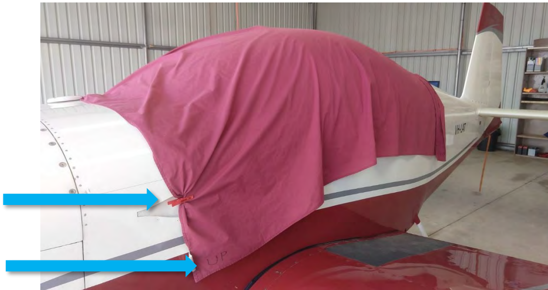
Figure 53 - Canopy cover secured with a peg on each side. Keep the cover the right way up to help protect the windshield.
