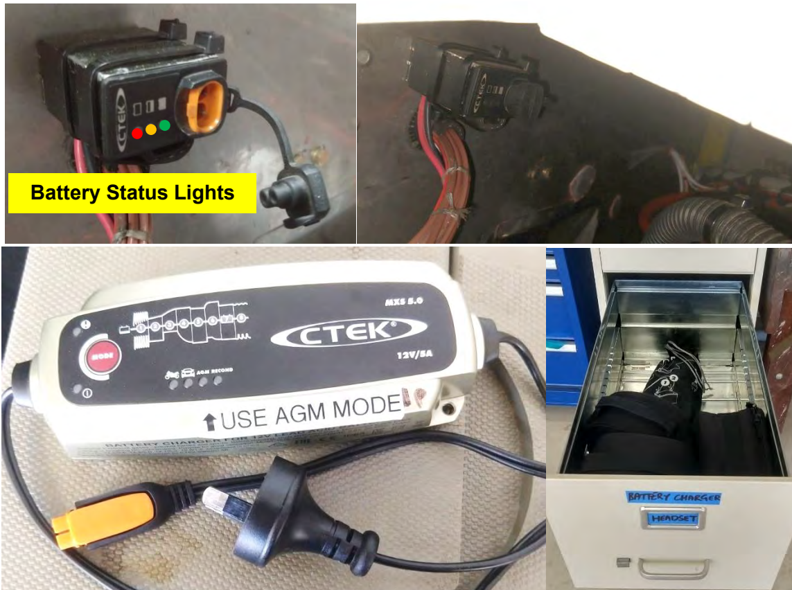
Figure 14 – TOP: Battery monitor and trickle charge connector located on the firewall. Accessible through the oil flap.
