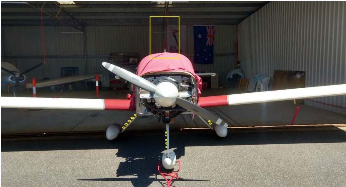
Figure 38 – Line the aircraft up nice and straight with the markings outside the hangar first. The wheels should be in line with the ground markings and the tail in line with the hangar support beam. Then go straight back (do not follow the curved pink dots inside the hangar)
